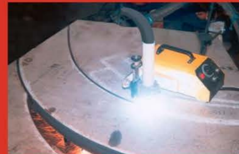
80 mm stainless steel cutting on circle cutting trolley
