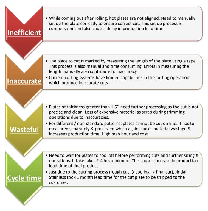
As a result, JSL was struggling with inefficiency, inaccuracy, wastage & production delays with this cutting technology & method added up with the additional cost of material handling, inventory & labour. That is the context in which Jindal Stainless began considering using robotic plasma cutting process to red hot plates.
