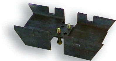
❶ Structural I beam with bolt holes cut on a Plazma robotic system
