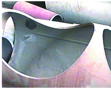
❶ A 3-dimensional pipe saddle, cut on the system
