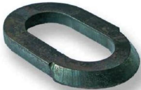
Beveling is done on plates most of the time for weld preparation. This was made either by using a hand torch or milling machine. With the hand torch method, the finish had a bad, uneven beveled edge. With the milling machine, we obtained excellent cut edges. But the time taken and cost involved was very high. With the RoboPlazma™, we have been able to achieve a high cut edge finish in shortest possible time. We have recently completed a number of export jobs with quality, in time delivery.
